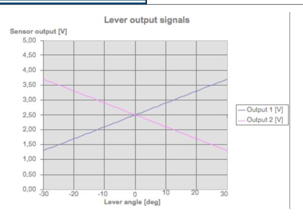
Output voltage is proportional to supply voltage. Defined output voltage above is specified with supply voltage  $\pm 5.0V \pm 1\%$ .
