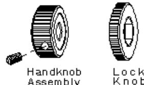
Sun offers a general purpose handknob with lock knob control for use in systems where frequent adjustments are necessary. The handknob components are added to the basic L control. Cartridges may be ordered in this configuration from Sun by specifying a K control in the model number. Sun kits for field conversion are also available.
