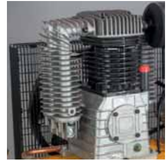
Pumping unit with large manifolds for better cooling of the compressed air.
