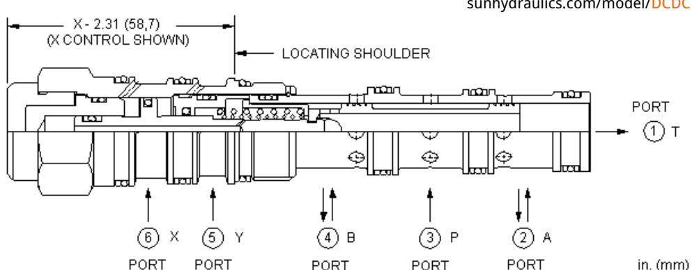
Three-position, 4-way directional cartridges are spring-centered, 6-port directional valves that can be configured from a choice of spool options. The supply port is port 3 and all ports will accept 5000 psi (350 bar). Capacity for these pilot-to-shift valves is dependent on the spool type specified.
