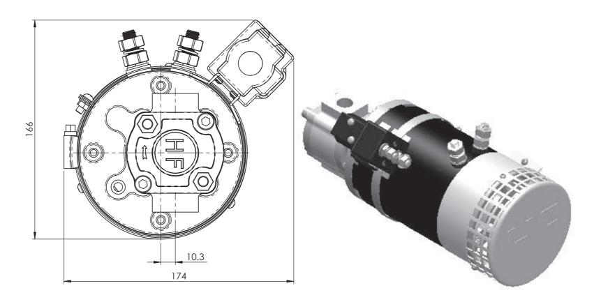
The DC motor is of \$2/\$3 duty, which can only be worked intermittently.
