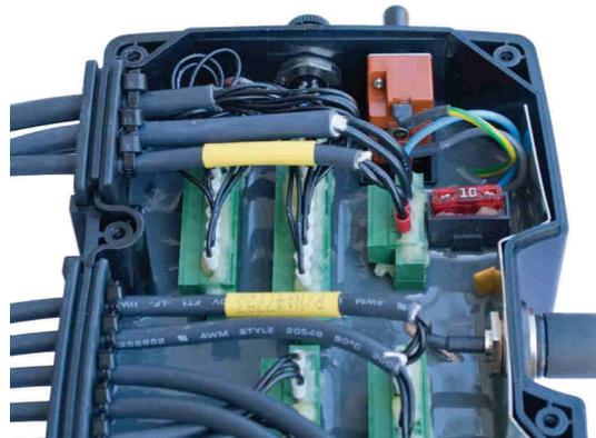
Figure 5.7 Cable orientation.
