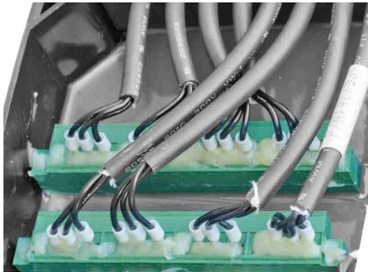
Figure 5.6 Applied grease.
