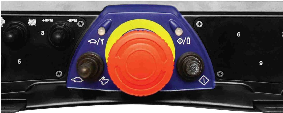
Figure 3.4 View of a stop function panel.
