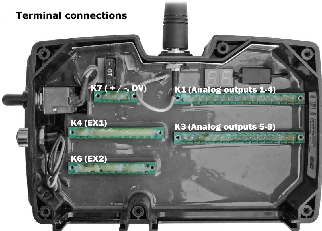
Figure 3.9 The figure illustrates inside terminal connectors for the standard Central Units type 2000 (Danfoss) and type 3000 (PWM).
