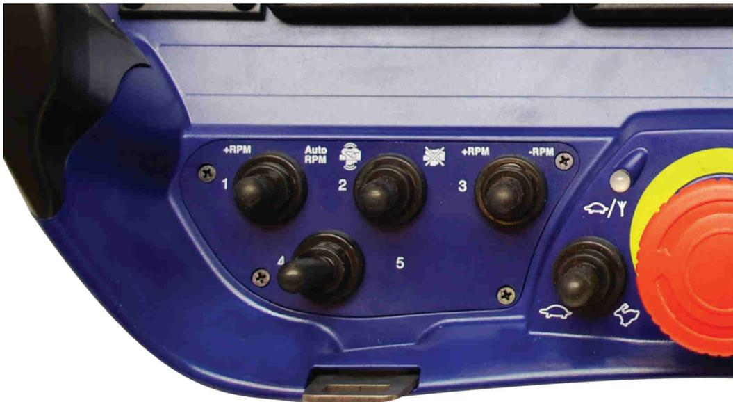
Figure 3.5 Left switch panel on MAXI PCU.
