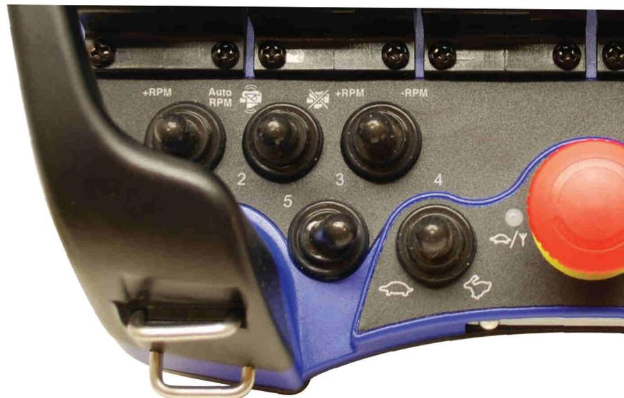
Figure 3.6 Left switch panel on MINI PCU.
