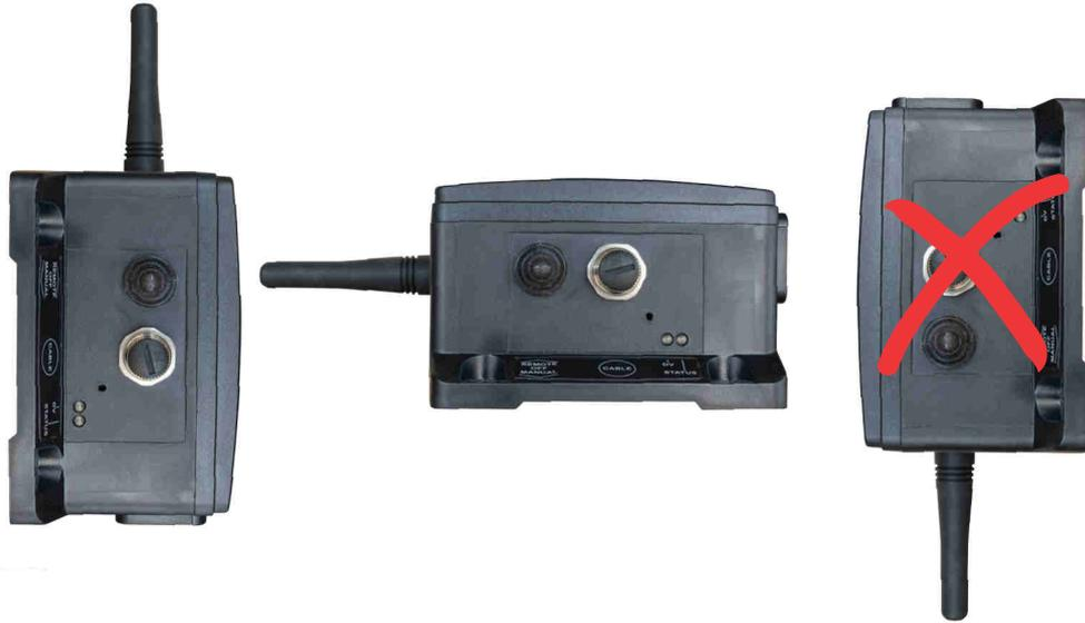
Figure 5.2 How to mount the Central Unit.
