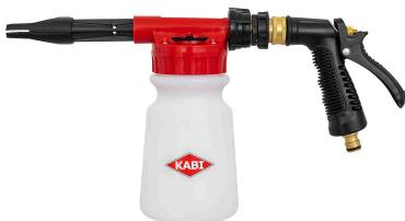
KABI Foam Gun - Low Pressure Foam gun for exposition, and cleaning with foam. Connects to a water hose and works with normal water pressure (2.5-6 bar). 0.9 litre transparent container. Foam nozzle can be rotated 90°. Robust trigger with brass quick coupling, for easy water supply. Integrated mixing ratio dial with 6 different mixing ratio settings.
