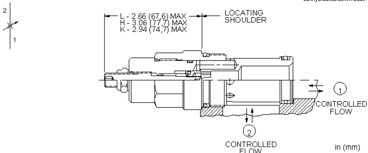
Needle valves are fully adjustable orifices used to regulate flow. They are infinitely adjustable from fully closed up to the maximum orifice diameter. They are not pressure compensated and may be used as flow controls or as shutoff valves.
