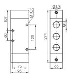
Weight 4200 g Minimum pilot pressure 3 bar
