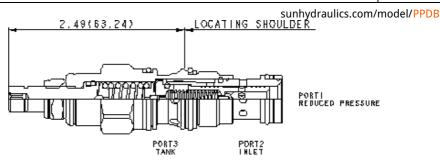
Pilot-operated, pressure reducing/relieving valves reduce a high primary pressure at the inlet (port 2) to a constant reduced pressure at port 1, with a full-flow relief function from port 1 to tank (port 3).
