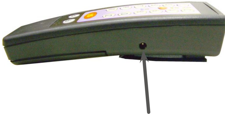
Battery charger connection
