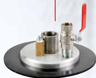
P/N 11/34 Membrane ø 310 mm with NBR seal ring and 45 mm ø suction tube adaptor (for drum internal ø 260 - 310 mm)
