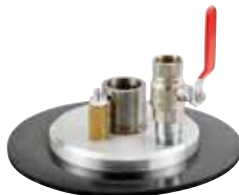
P/N 11/34 Follower plate ø 310 mm with NBR seal ring and suction tube adaptor ø 45 mm (for drum internal ø 260 - 310 mm)
