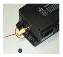
3) Switch on the transmitter in ASSIGN mode: holding down the keys 3 and 4, press and release the STOP button.
