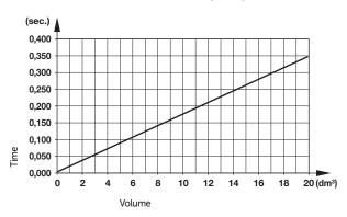
Note: Graphs provided with silencer fitted directly on capacity. Restriction between capacity and silencer will introduce additional time.
