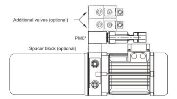
Note: Recommended tightening torque for M8 bolts: 16 Nm. Attention! Do not use tie-rods less than 8.8.
