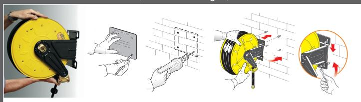
The solid and compact bracket is provided with four slotted mounting holes for easy and safe installation. Using the template supplied with the hose reel it's easier to mark plugs holes for hose reel fixing.
