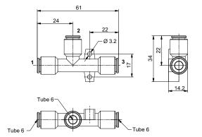
Single stage generators, robust and reliable, with compact dimensions and suitable for applications that need the required degree of vacuum to be reached quickly with limited air flows. Operating on the Venturi principle they have the vacuum connection orthogonal to the axis of supply and outlet. They can be connected directly to the suction cups and/or suction cup holder and can be applied in any position.
