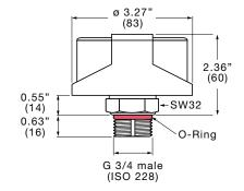
Dimensions are for general information only, all critical dimensions should be verified by requesting a certified print. Dimensions are in inches/(mm)
