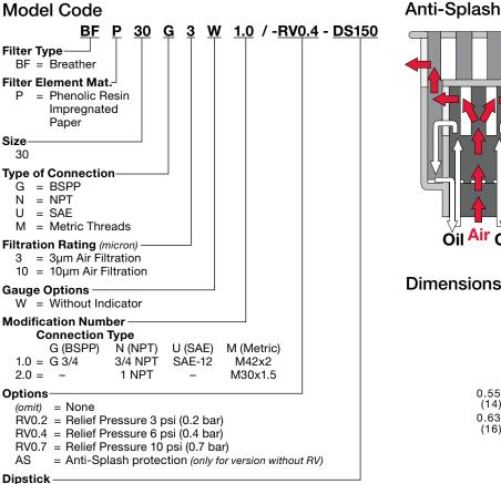
. DS# = Dipstick (Length follows DS in millimeters) minimum quantities apply
