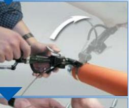
Place band in tool, push down on gripper with thumb, tension clamp by turning handle. Maximum tension is reached when band stops moving through buckle. When required tension has been applied, roll tool over buckle, at the same time reversing handle carefully approx.  $\frac{1}{2}$  turn to avoid breakage. There is no loss of tension, if handle is not reversed too much.
